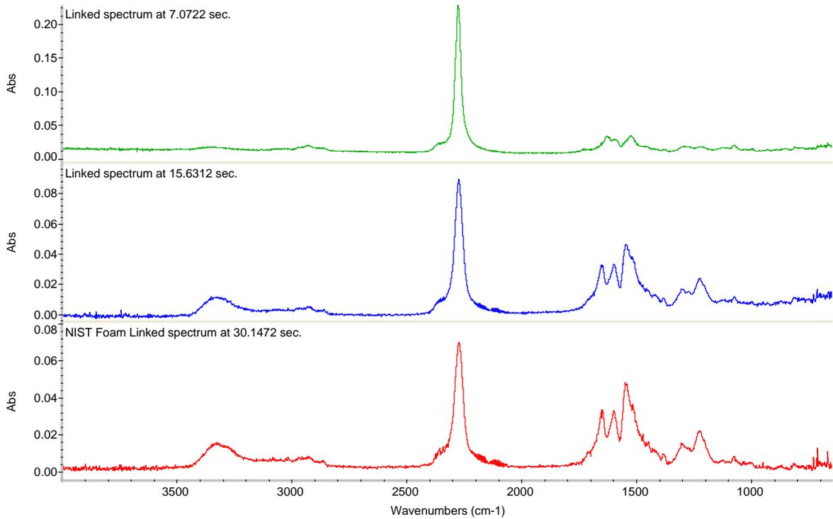
Figure 14. Infrared spectrum of foam pyrolysis progression.
