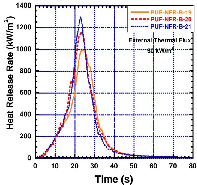
Figure D-12. Heat Release Rate versus Time for Polyurethane Foam Exposed to 60 kW/m<sup>2</sup> of External Heat Flux (PUF-NFR-B). Samples PUF-NFR-B-19, PUF-NFR-B-20, and PUF-NFR-B-21.
