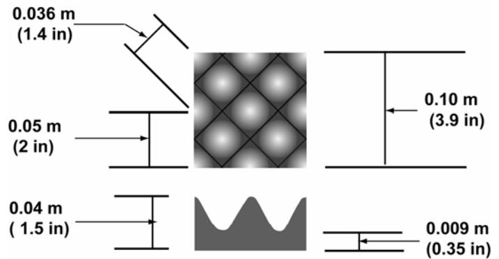
**Figure D-6. Photograph and Dimensioned Diagram of Non Fire Retardant Foam Lot B (PUF-NFR-B).**
