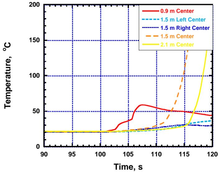
Figure F-16b. Temperatures versus Time for Single Gerb Discharged at 45 Degrees in Plane Perpendicular to Wall.
