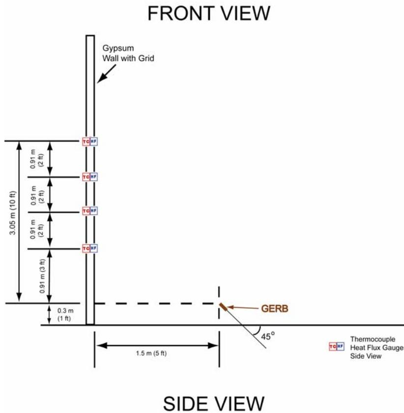
Figure F-7. Instrumentation Diagram for a Single Gerb at 45 degrees and in a Plane Perpendicular to Wall.
