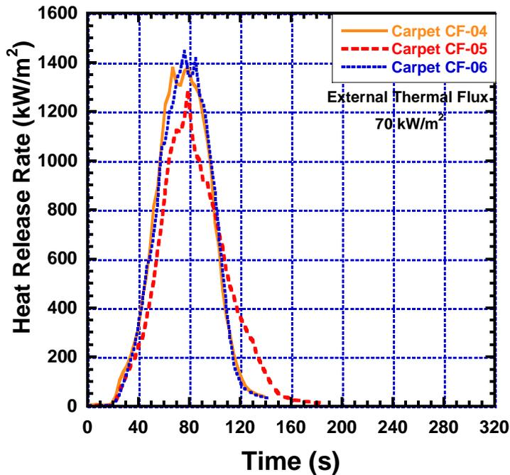
Figure D-23. Heat Release Rate versus Time for Carpet Sample Exposed to 70 kW/m<sup>2</sup> of External Heat Flux (CF). Samples are CF-04, CF-05, and CF-06.
