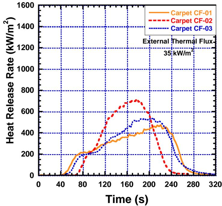
Figure D-22. Heat Release Rate versus Time for Carpet Sample Exposed to 35 kW/m<sup>2</sup> of External Heat Flux (CF). Samples are CF-01, CF-02, and CF-03.
