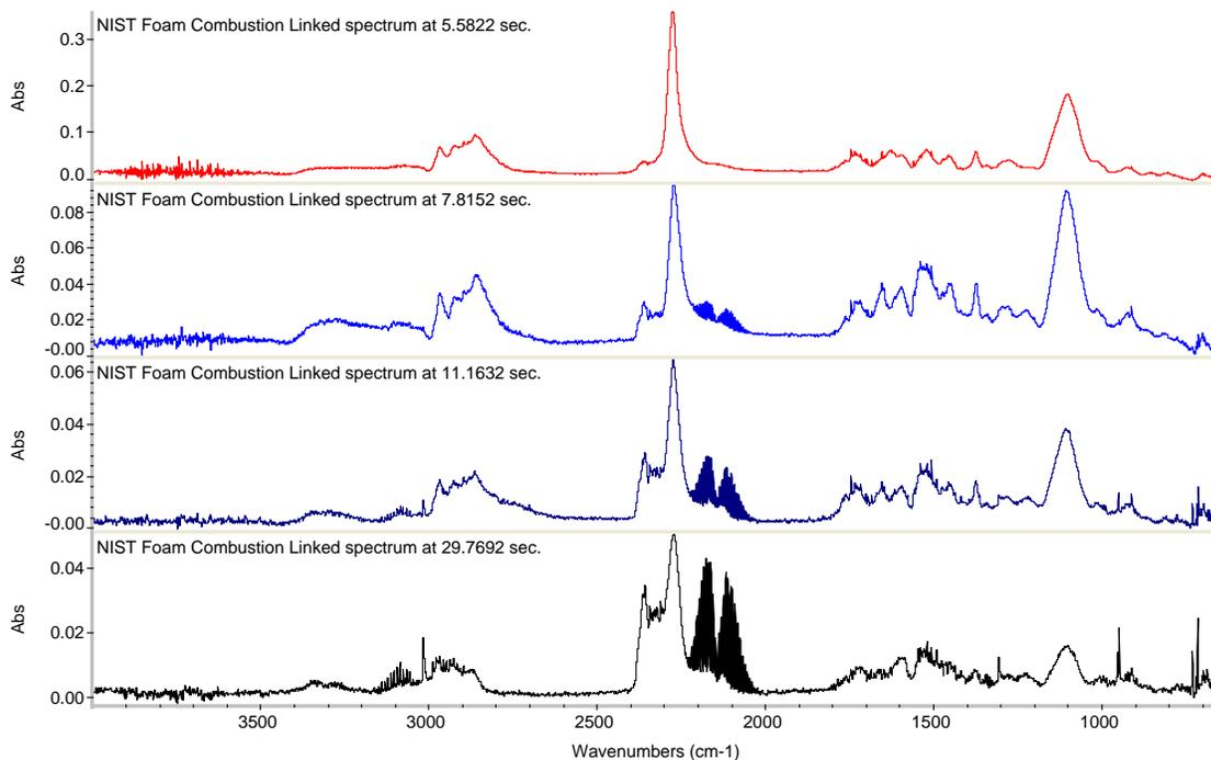
Figure 18. Infrared spectrum of foam combustion progression. Note the growth of the carbon monoxide peak (centered at  $2150\text{ cm}^{-1}$ ) as the combustion progresses from 5 to 30 seconds. The isocyanate compound peak ( $\sim 2270\text{ cm}^{-1}$ ) dominates each spectrum. The polypropylene peak ( $\sim 1100\text{ cm}^{-1}$ ) is decreasing showing that the oily polypropylene glycol compound is being consumed as the combustion progresses.
