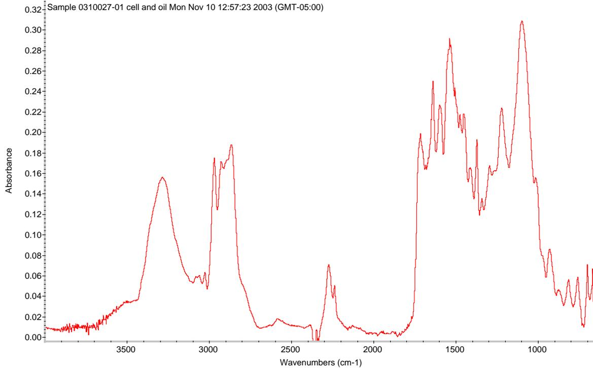
Figure 3. Infrared spectrum of sample unburned gray foam.
