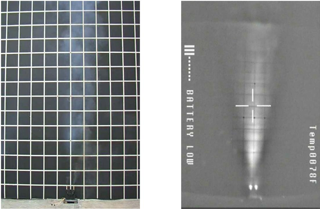
Figure F-22. Standard Video and Infrared Video Images of Gerb Discharge at 16 seconds.
