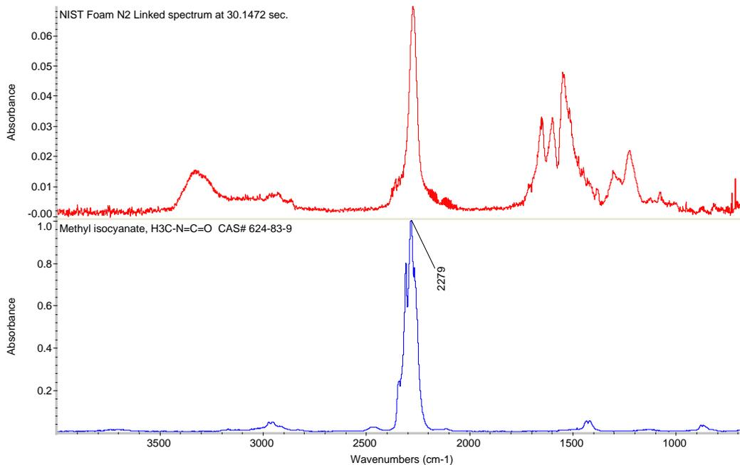
Figure 12. Infrared spectrum of sample pyrolyzed foam (top). Best library match is methyl isocyanate (peak ~2270 cm<sup>-1</sup>). This is a match to a class of isocyanate compounds. Methyl, Propyl, and even Butyl isocyanate have spectra that cannot be distinguished at this resolution.
