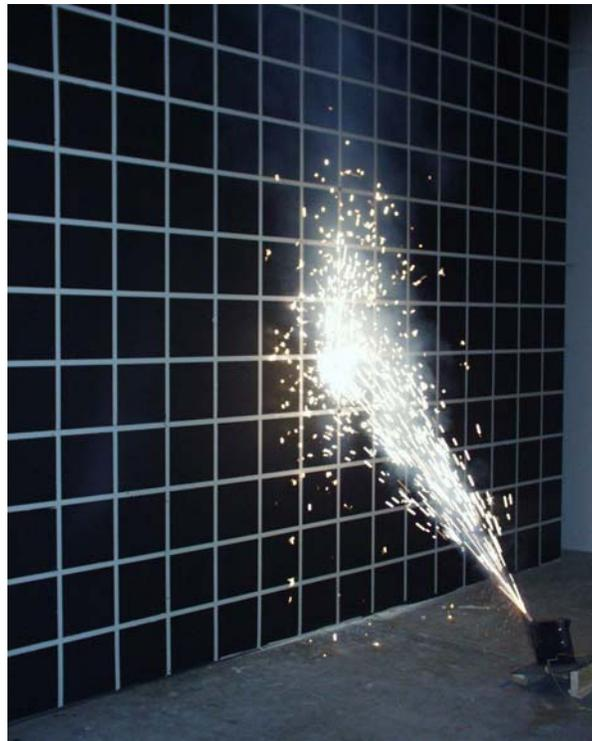
**Figure F-4. Single Gerb at 45 degrees and in a Plane Perpendicular to Wall.**
