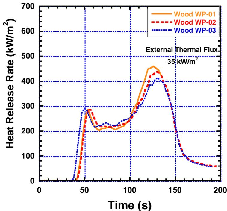
Figure D-19. Heat Release Rate versus Time for Wood Paneling Exposed to  $35 \text{ kW/m}^2$  of External Heat Flux (WP). Samples are WP-01, WP-02, and WP-03.
