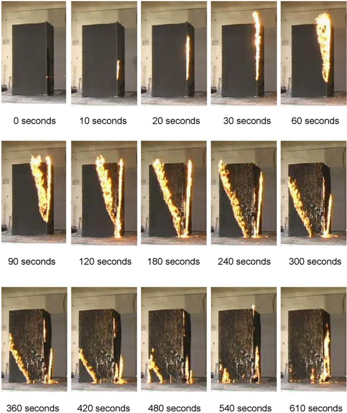
**Figure E-5. Flame spread over polyurethane foam covered panels, external corner configuration.**
