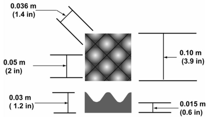
**Figure D-5. Photograph and Dimensioned Diagram of Non Fire Retardant Foam Lot A (PUF-NFR-A).**
