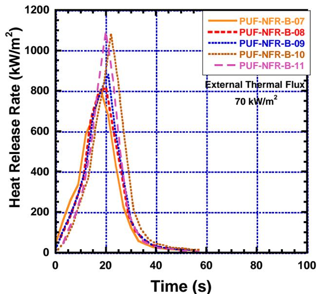
**Figure D-13. Heat Release Rate versus Time for Polyurethane Foam Exposed to 70 kW/m<sup>2</sup> of External Heat Flux (PUF-NFR-B). Samples PUF-NFR-B-07, PUF-NFR-B-08, PUF-NFR-B-09, PUF-NFR-B-10, and PUF-NFR-B-11.**
