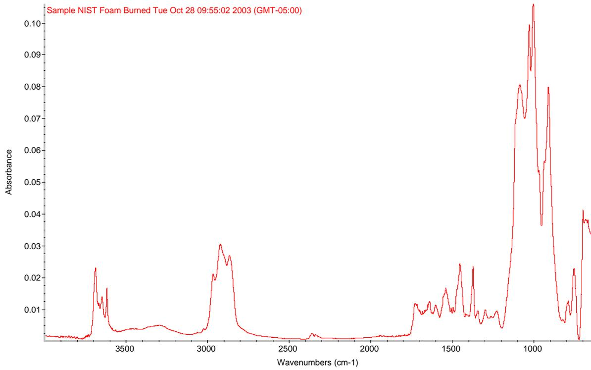
Figure 8. Infrared spectrum of sample foam adhesive.
