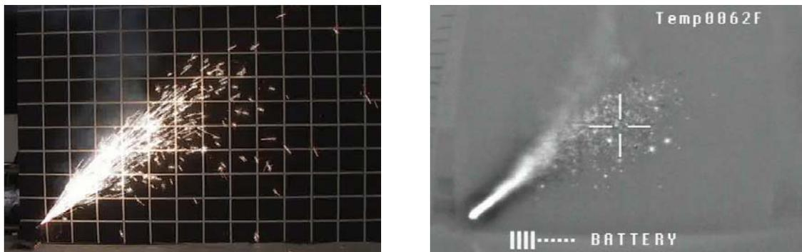
Figure F-9. Standard Video and Infrared Video Images of Gerb Discharge at 2 s.
