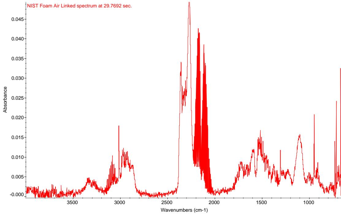
Figure 15. Infrared spectrum of foam combustion in air.
