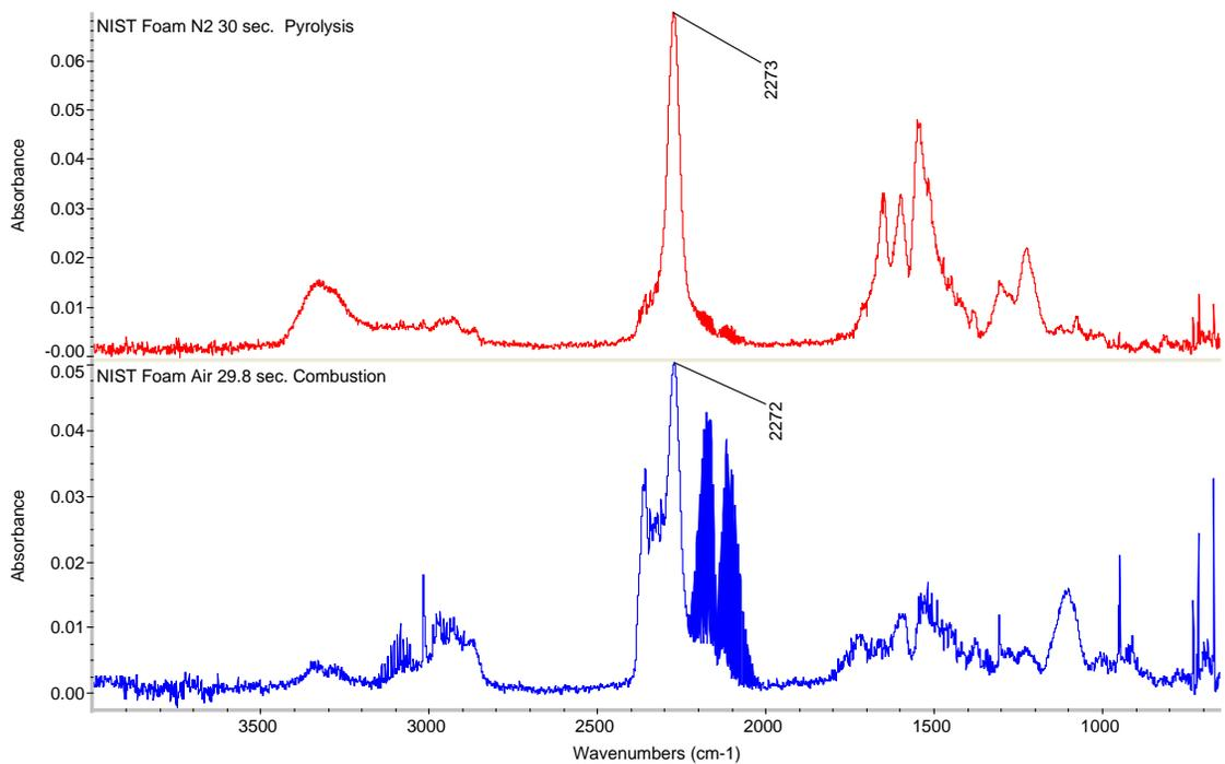
Figure 2. Infrared spectrum of foam pyrolysis gases (top) and combustion gases (bottom). The dominate peak in each spectrum is the peak at  $\sim 2270\text{ cm}^{-1}$ . This peak most closely matches isocyanate compounds (see figure 3). The related isocyanide compounds are not a good match (see figure 4) because their absorbance is too far from  $2270\text{ cm}^{-1}$ .
