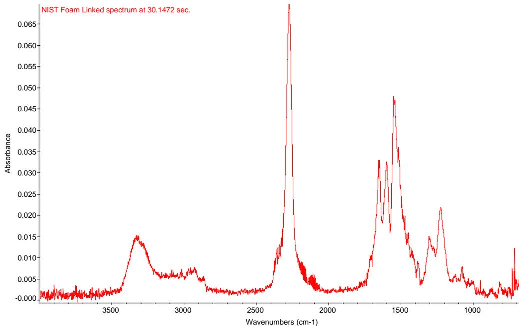
Figure 11. Infrared spectrum of foam pyrolysis. The isocyanate peak 2270 cm<sup>-1</sup> is from a class of compounds with the general formula H<sub>x</sub>C<sub>x</sub>HNO. These compounds are very toxic.
