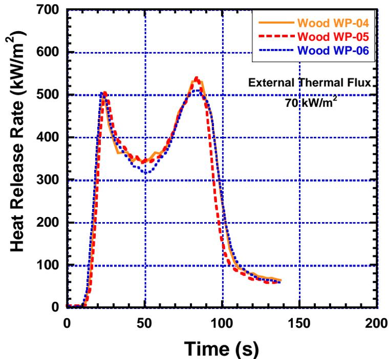
**Figure D-20. Heat Release Rate versus Time for Wood Paneling Exposed to 70 kW/m<sup>2</sup> of External Heat Flux (WP). Samples are WP-04, WP-05, and WP-06.**
