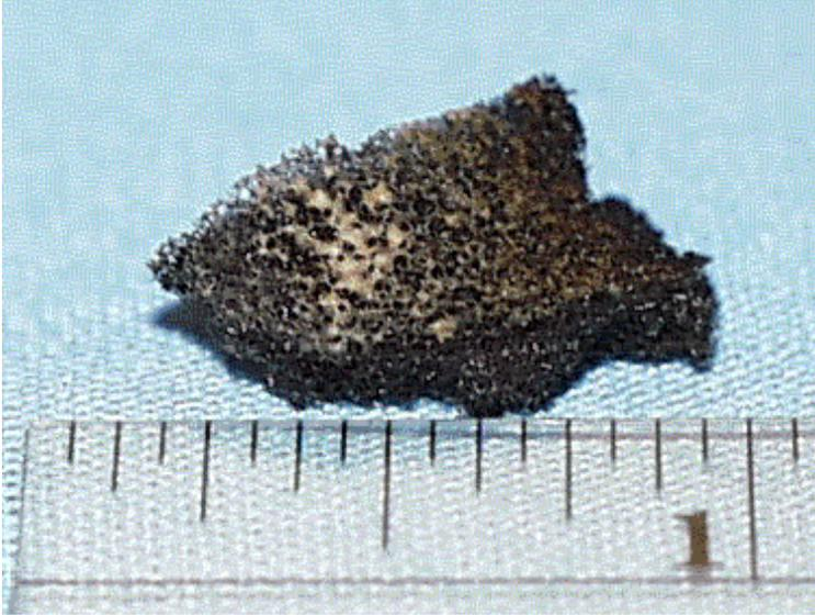
Figure 7. Sample 0310027-02 piece1 foam with adhesive.
