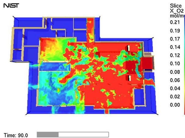
Figure 9. Oxygen volume fractions at 0.6 m (2 ft) above the floor at 90 s
